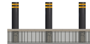
Painted Bollard and Flat top with Banding
