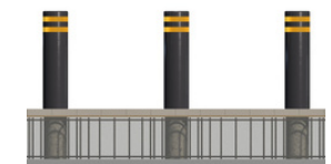
Bollard and Painted Flat top Banding
